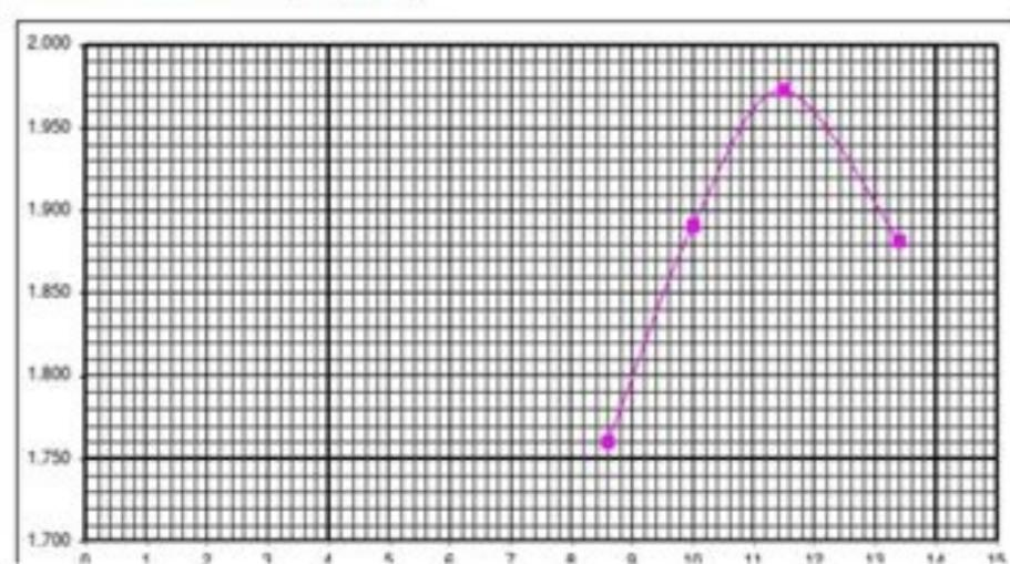
The results of a standard Proctor test are given in the following table. Determine the maximum dry density ( $\text{kg/m}^3$ ) of compaction and the optimum moisture content.
